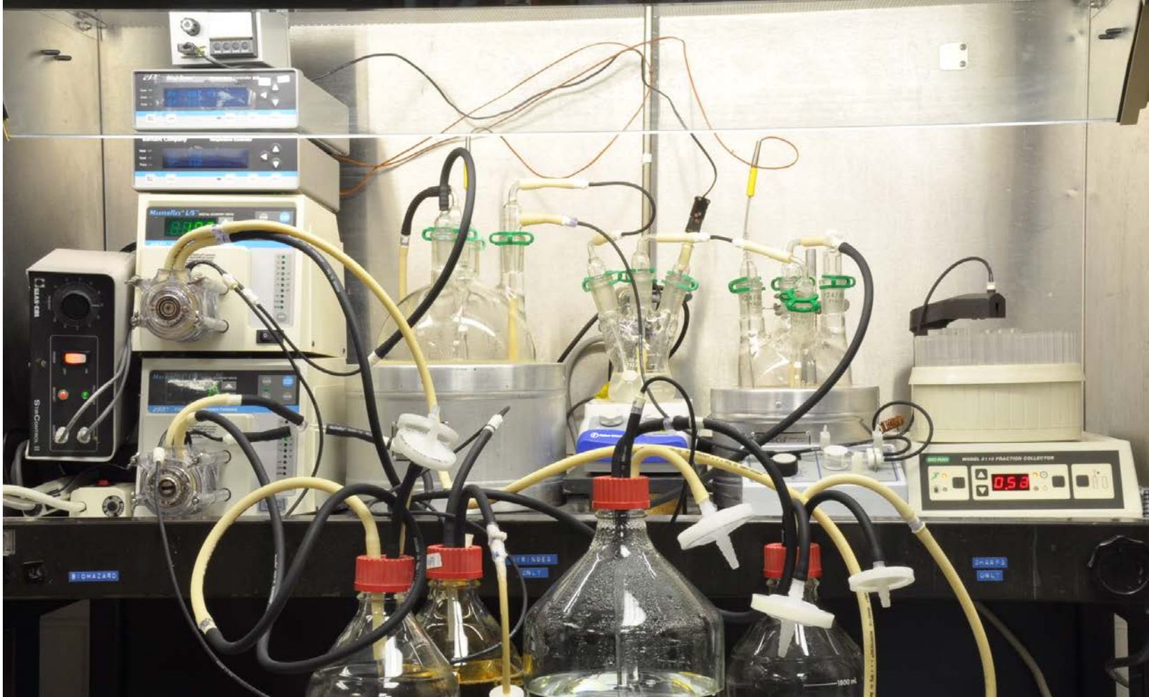
Figure 3. Picture of the HSC illustrates spatial and organizational challenges. This picture shows long inter-reactor path lengths and accommodations to mix water and medium concentrate by pump, features which were eliminated in later revisions. Note that HS 1 in this picture is an Erlenmeyer flask, while it is diagramed as a round bottom flask in Figure 2.
